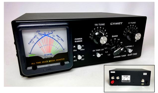
Max Power: 300W (SSB) Tunes dipoles, verticals, mobile whips, long wires and other antenna designs in all bands between 1.8MHz and 50Mhz Input impedance: 50 Ohm Output impedance: 10 - 600 Ohm Cross needle meter displays forward power, reverse power, and SWR simultaneously Voltage required for meter light: DC 11V - 15V, 250mA approximate Weight: 6 lb approximate Dimensions: 10 x 4 x 8 inches approximate
