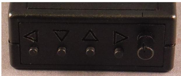
This is the **controls** end of your PicoKeyer. The speed control knob is on the right, the memory/setup pushbuttons are on the left. The triangle symbols ◀, ▼, ▲ and ▶ are used with the setup menu system. The buttons are not marked with numbers, but are numbered from 1 through 4 from left to right for message memories.
