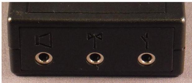
This is the **connections** end of your PicoKeyer. The center jack is for your paddles (input); the right hand jack is the on/off output for keying your transmitter or transceiver (output). The left hand jack is a low power audio output that can be used for ear buds or headphones.
